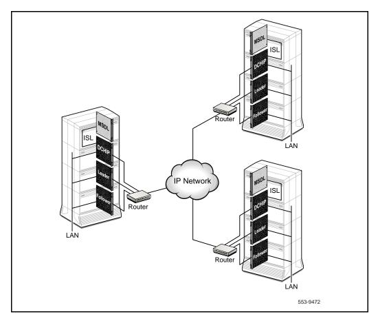
ISDN signaling between the Meridian 1 and the ITG ISL Trunk supports the delivery of Calling Line Identification (CLID) and feature messaging. ISL DCH signaling provides the necessary signaling connection over which data, including CLID and feature-specific messaging, can be passed.
